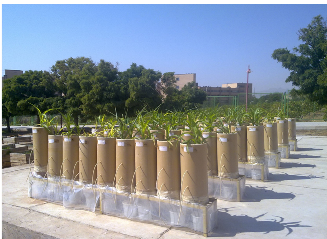
Figure 1. The layout of the soil column experiments conducted in 2014 at the College of Agriculture, Isfahan University of Technology.
