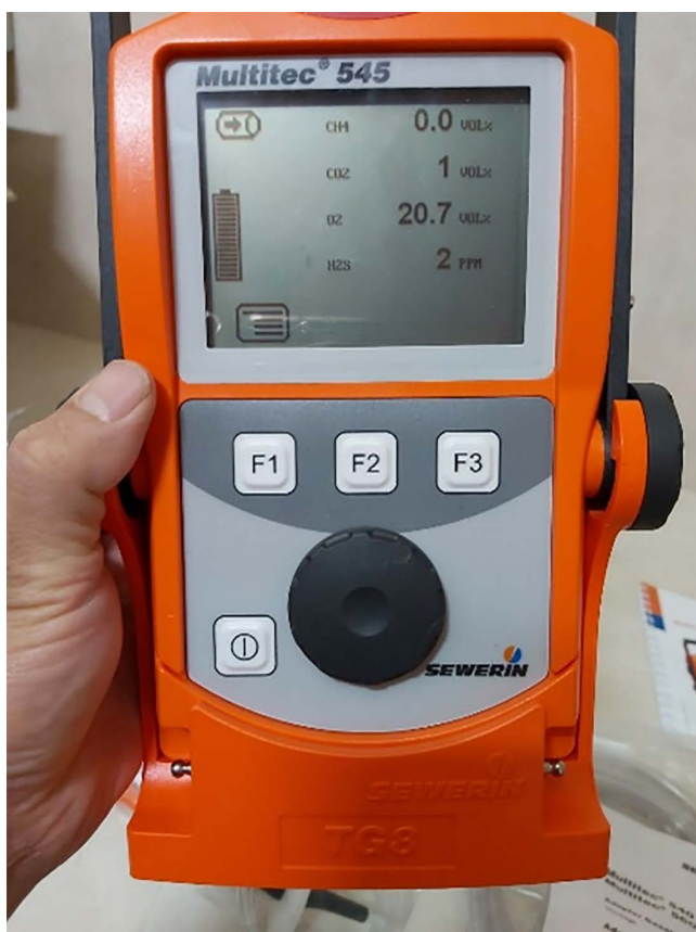
Fig 3. MultiTech 545 gas analyzer used for biogas composition analysis.
