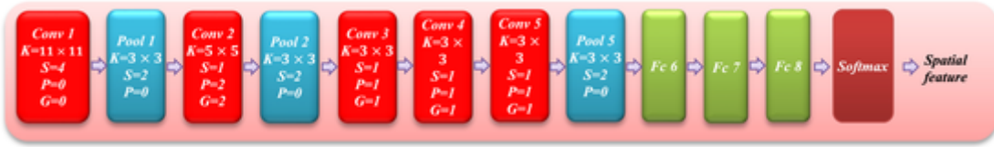
Fig. 2. The main layers of the standard AlexNet [41], consists of 5 convolutional layers (colored red), 3 pooling layers (colored blue), 3 fully connected layers (colored green) and finally one Softmax layer (colored brown).
