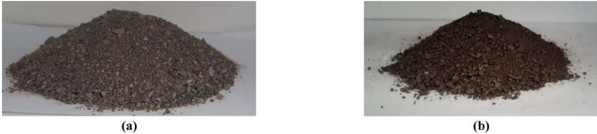
Fig. 1. Sample of fine aggregates: (a) Natural sand, (b) waste foundry sand.
