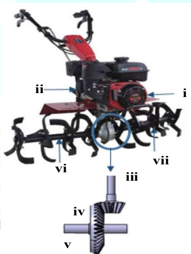
Fig. 1. The two-wheel tractor, i engine, ii gearbox, iii umbrella gear shafts, iv umbrella gear (cone gear), v rotary output shaft, vi left rotary axle, vii right rotary axle
