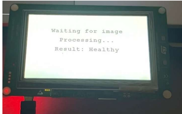
Figure 4: Result of the model's prediction on LCD, which occurs simultaneously with UART.
