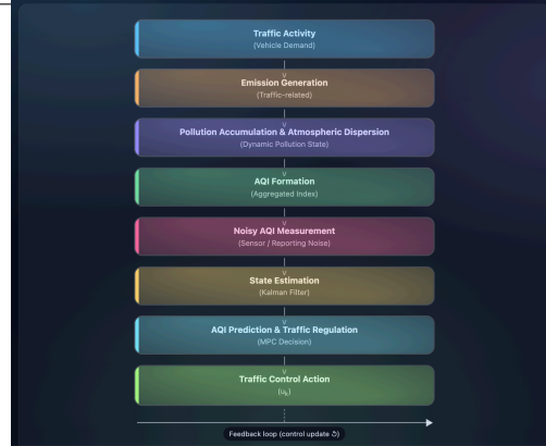
FIGURE 1. Conceptual flowchart illustrating how traffic activity influences AQI dynamics through emissions
