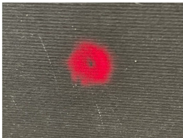
Fig. 8 The separated Laguerre–Gaussian beam from the diffraction pattern of a fork-shaped grating with a topological charge equal to 1 by an adjustable aperture
