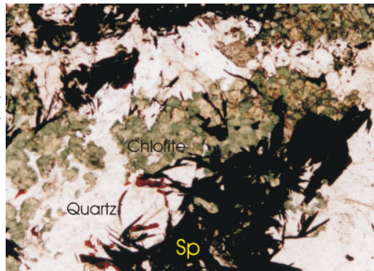
Fig. 3 Photomicrograph shows specularite (Sp) having bladed forms formed first then it followed by quartz and chlorite.
