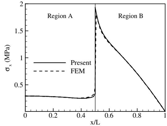
Fig. 3. Distribution of in-plane normal stress  $\sigma_x$  at  $z = h/4$  in  $90^\circ$  ply in region A and  $0^\circ$  ply in region B.
