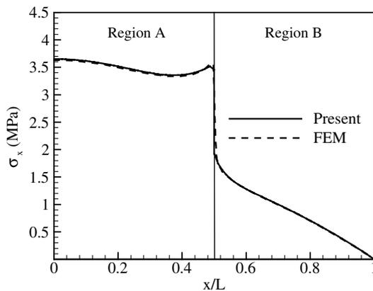
Fig. 2. Distribution of in-plane normal stress  $\sigma_x$  at  $z = h/4$  in  $0^\circ$  plies in regions A and B.
