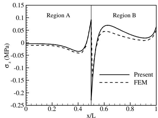
Fig. 5. Distribution of interlaminar normal stress  $\sigma_z$  at the middle plane.
