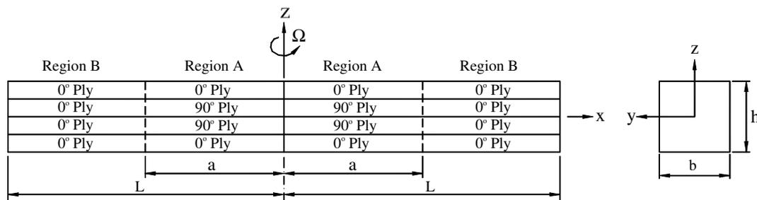
Fig. 1. The geometry of problem with a  $[0^\circ/90^\circ]_s$  laminated beam (region A) in transition to  $[0^\circ/0^\circ]_s$  laminated beams (regions B).
