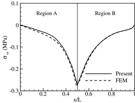
Fig. 6. Distribution of interlaminar shear stress  $\sigma_{xz}$  at  $z = h/4$  along the  $0^\circ/90^\circ$  interface in region A and along the  $0^\circ/0^\circ$  interface in region B.
