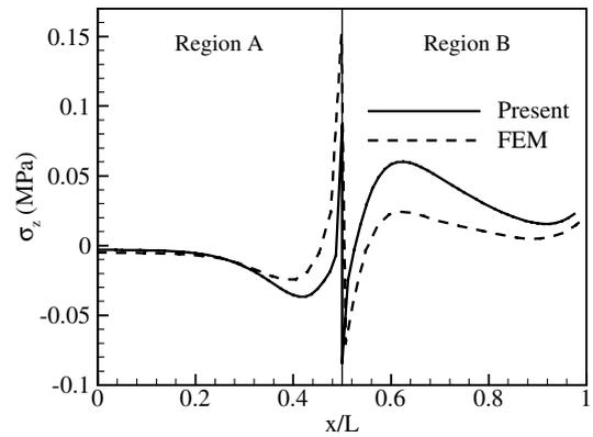
Fig. 4. Distribution of interlaminar normal stress  $\sigma_z$  at  $z = h/4$  along the  $0^\circ/90^\circ$  interface in region A and along the  $0^\circ/0^\circ$  interface in region B.
