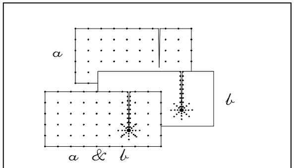
Figure 1. Node distribution in an overlay made of field nodes (a) and crack tip nodes (b).
