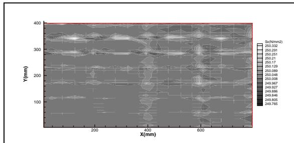
Figure 1. Distribution of  $\sigma_x$  in the Elastoplastic uniaxial stretch of a rectangular thin plate.
