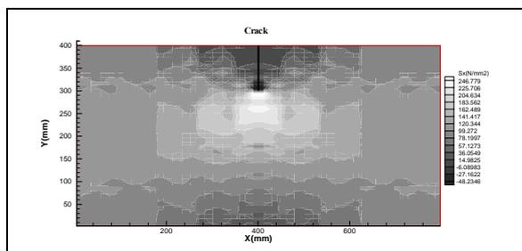
**Figure 5. Equivalent stress ( $\bar{\sigma}$ ) developed in a plate having an open crack and loaded in both sides**
