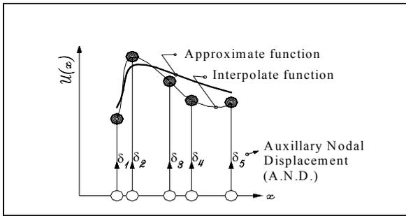
**Figure 1. A comparison between the concepts of the interpolation as used in FEM and the approximation as used in EFG.**
