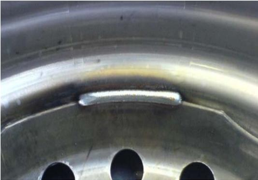
Figure 10 - an example of a valid weld on automobile wheel
