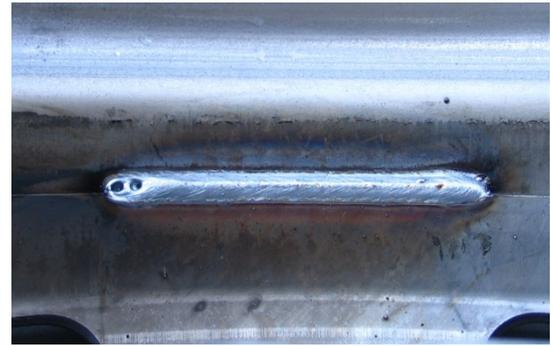
Figure 11 - an invalid weld with cavity
