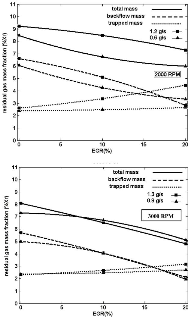
Fig.3.Development of residual gas mass fraction for different EGR ratio in an IDI diesel engine at 1500, 2000 rpm and 3000 rpm under two fuel injection rates.(OF=0.93)
