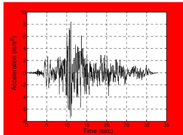
Figure 2: Tabas earthquake acceleration spectrum
