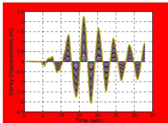
Figure 8: Structure time response without TMD for dense soil
