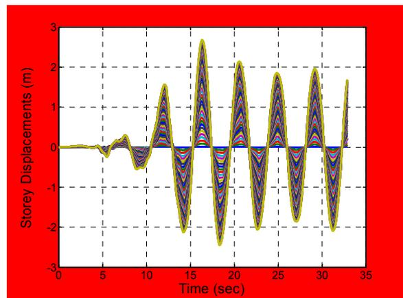
Figure 6: Structure time response without TMD for medium soil
