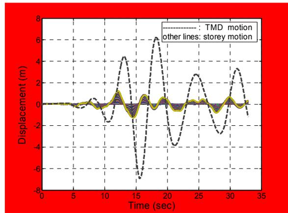
Figure 5: Structure time response with TMD for medium soil
