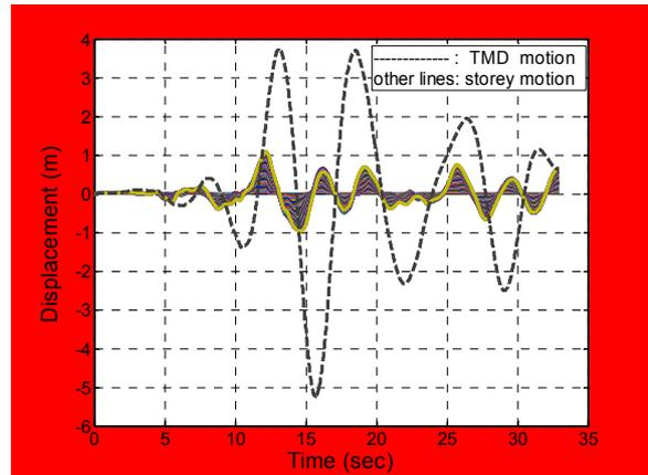
Figure 7: Structure time response with TMD for dense soil
