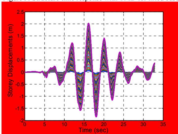
Figure 10: Structure time response without TMD for fixed base
