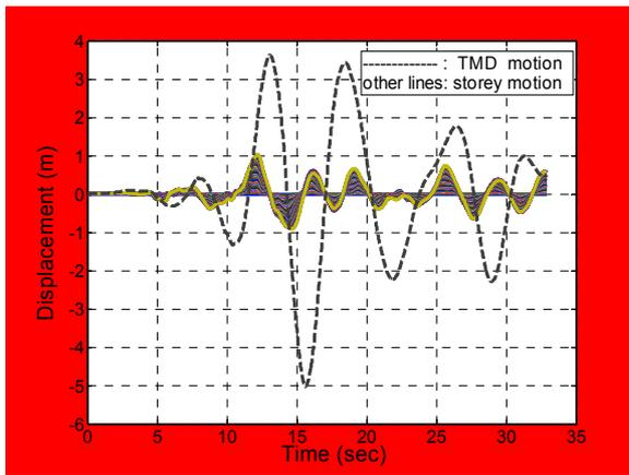
Figure 9: Structure time response with TMD for fixed base
