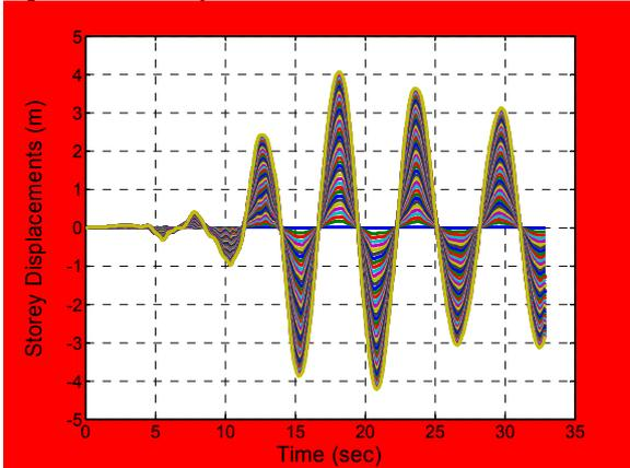
Figure 4: Time response of structure without TMD for soft soil
