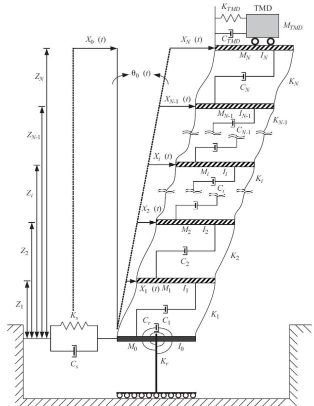
Figure 1: Shear building configuration
