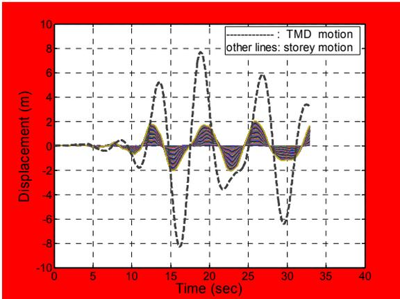
Figure 3: Time response of structure with TMD for soft soil
