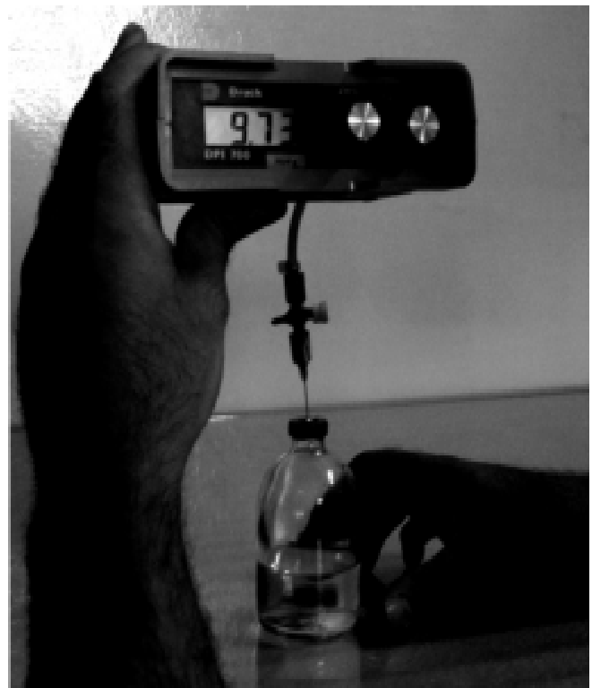
Figure 1. Pressure gauge and modified B Braun plastic stopcocks-3 way used for pressure measurements
