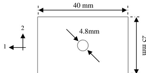
Fig. 2. Specimen in detail accompanied with dimensions
