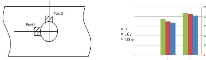
Fig5, (a) overall orientation of the elements in plate and mandrel; (b) The magnitude of compressive residual stress on points 1 and 2 for different mandrel speeds
