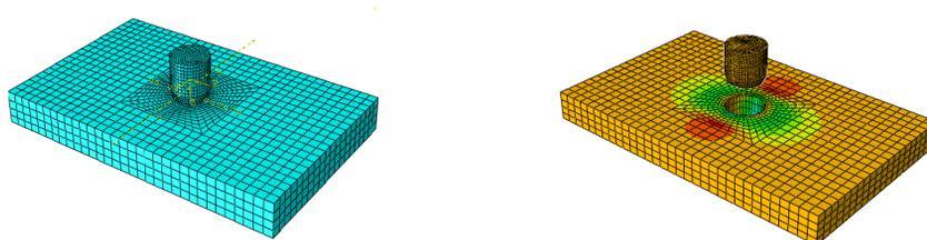
Fig.3. (a) overall orientation of the elements in plate and mandrel; (b) compressive residual stress distribution around cold expanded hole
