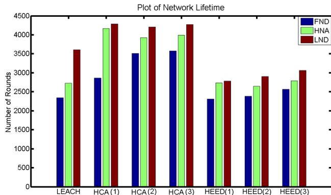
Figure 5. The comparison of different definitions of network lifetime in HCA, LEACH and HEED protocols with different communication costs: (1) node degree, (2) 1/node degree, and (3) AMRP.
