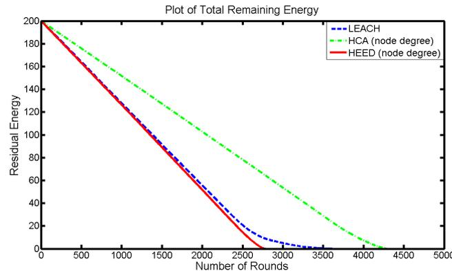
Figure 6. The comparison of total remaining energy in HCA, LEACH and HEED protocols with node degree communication cost.
