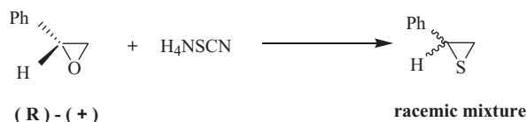
Scheme 2. Conversion of optically active (R) - (+) styrene oxide to a racemic mixture of styrene episulfide.
