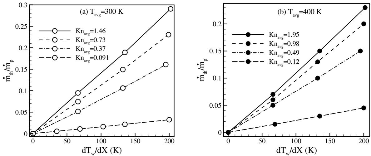
**Figure 4.** Non-dimensional thermal mass flow rate as a function of wall temperature gradient at different Knudsen numbers.
