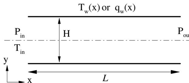
**Figure 1.** Micro/nanochannel geometry and imposed boundary conditions.
