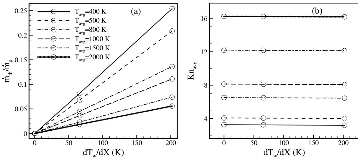
**Figure 6.** Thermal creep effects at high flow rarefaction and different flow temperature values; a) thermal mass flow rate and b) average Knudsen number.
