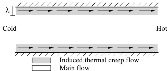
**Figure 3.** Thermal creep flow induced by wall temperature gradients.
