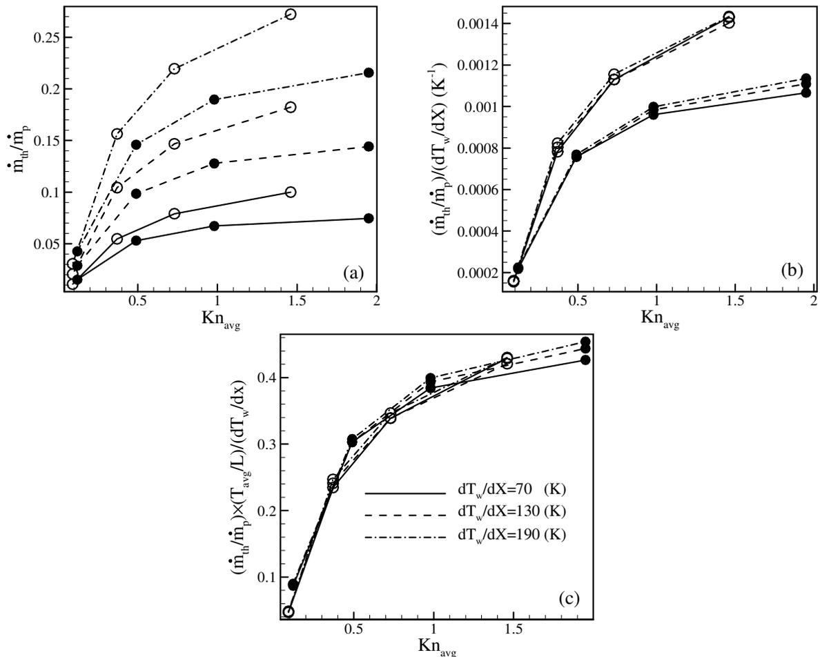
**Figure 5.** Thermal mass flow rate as a function of flow average Knudsen number, a) non-dimensional thermal mass flow rate, b) non-dimensional thermal mass flow rate independent from wall temperature gradient values, and c) non-dimensional thermal mass flow rate independent from wall temperature gradient and bulk flow temperature values. (White and black symbols denotes  $T_{avg} = 300$  and  $400$  K, respectively)
