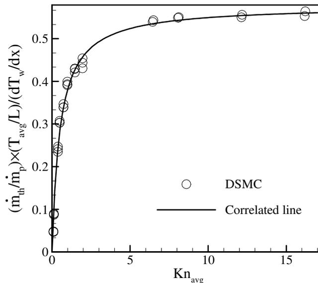
**Figure 7.** Thermal mass flow rate versus flow rarefaction from slip to free molecular regime.
