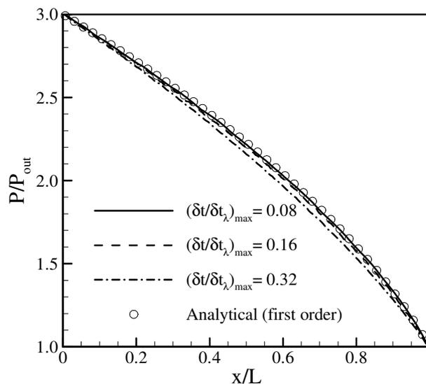
**Figure 2.** Pressure distribution along the channel for various DSMC time step values.
