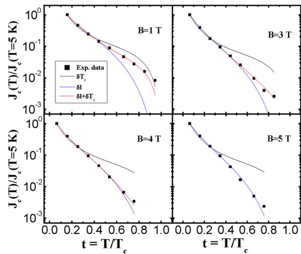
FIG. 2. Temperature dependence of the normalised measured current density  $J_c$  at magnetic fields of 1, 3, 4, and 5 T. The solid lines are the theoretical curves obtained based on the model of the  $\delta l$  (blue curves) pinning mechanism, the model of the  $\delta T_c$  (black curves) pinning mechanism, and the coexistence of both (red curves) pinning mechanisms.
