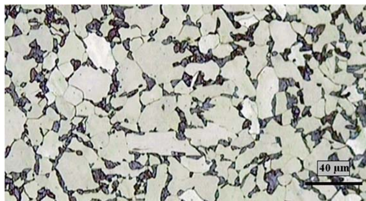
Figure 2- Dual phase microstructure of specimen intercritically annealed at 782°C with 28% of martensite
