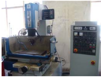
Fig 2 : Die-sinking EDM machine used for experiments
