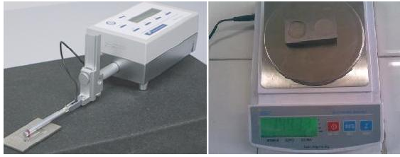
Fig 3 : Digital surface roughness tester and electronic balance
