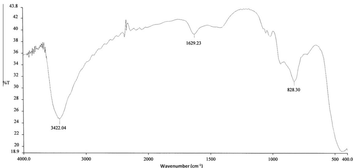
Fig. 5. FT-IR spectrum of prepared ZnO NPs with 0.4 g of HPW at 1 h stirring time.
