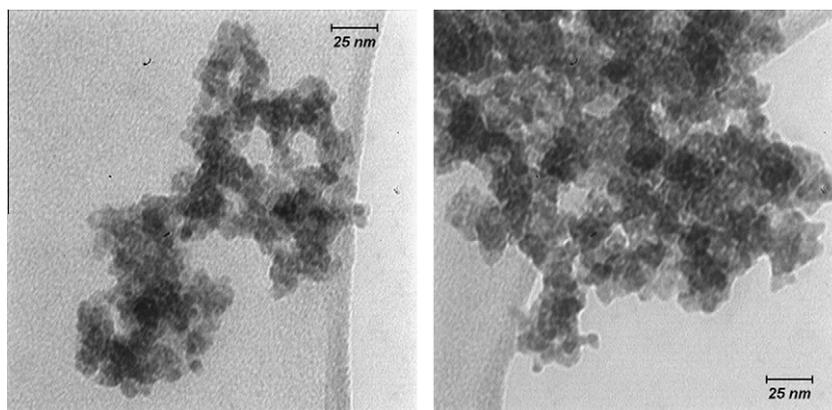
Fig. 4. TEM images of prepared ZnO NPs with 0.4 g of HPW at 1 h stirring time.
