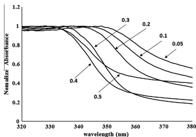
Fig. 2. Effect of HPW amount on UV-vis absorption spectra of prepared samples.
