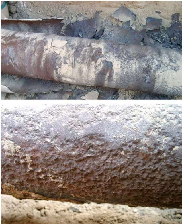
Figure 3 First HVG region of AL65 pipeline and the shape of corrosion
