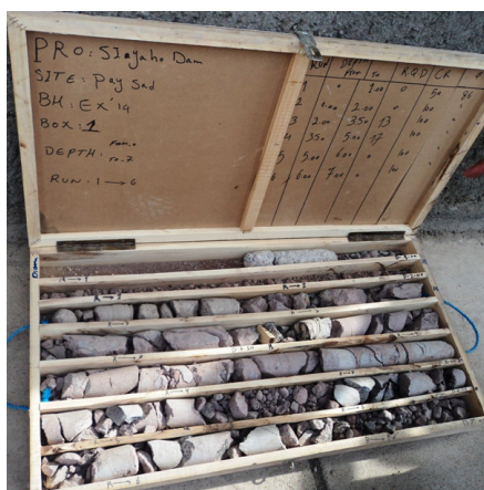
Figure 1. Core barrel samples in Exploration borehole (EX 14 ).
