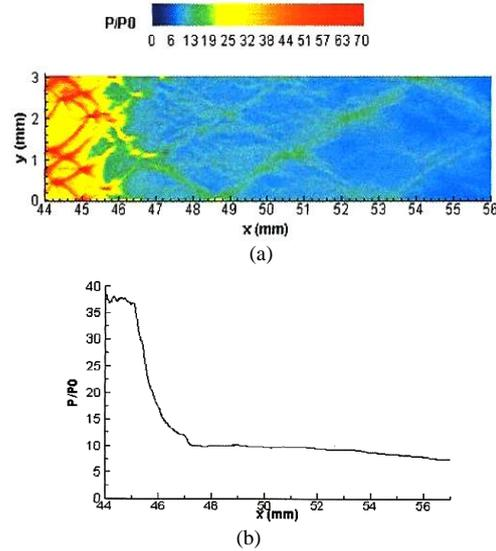
Fig. 4. Maximum pressure plot of the standard setup. The particle cloud is a belt of particles evenly distributed between  $x = 45\text{mm}$  and  $x = 47\text{mm}$ , and initial particle volume fraction 0.1%. (a). Maximum pressure for the standard setup, averaged in the y- dimension (b).
