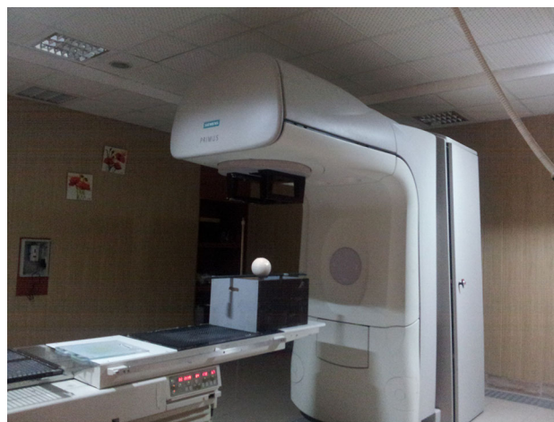
Fig. 2 Irradiation of Bonner sphere with 15 MV linac
