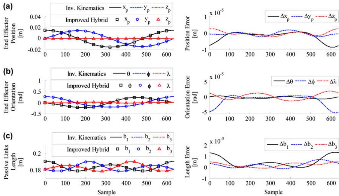
Figure 8. Improved hybrid method versus inverse kinematics solutions for 3-PSP robot. (a) Position of center of star platform, (b) orientation of star platform, and (c) passive links lengths.
