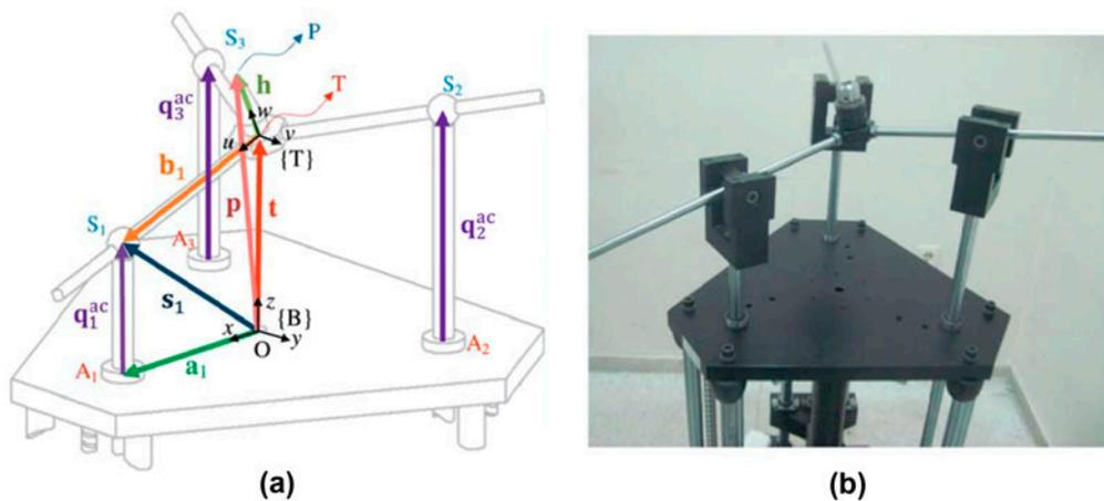
Figure 5. Required parameters for kinematic description of 3-PSP parallel robot [23].
