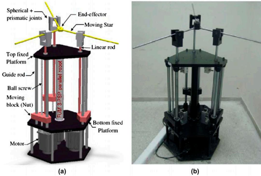
Figure 4. Spatial 3-PSP parallel robot: (a) CAD model and (b) physical model [22].
