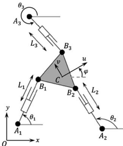
Figure 3. The 3-RPR parallel robot [20].
