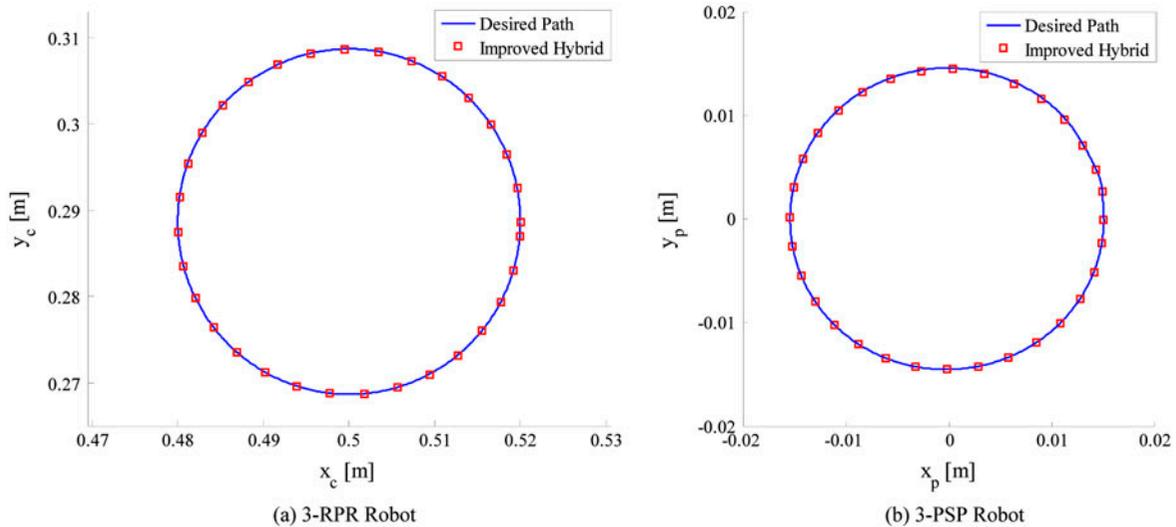
Figure 6. Evaluating the improved hybrid method in a circular path for (a) 3-RPR robot (b) 3-PSP robot.
