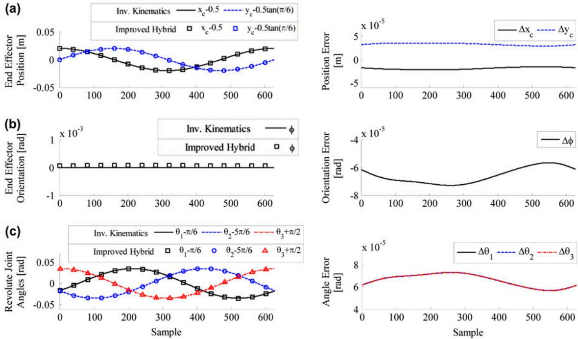
Figure 7. Improved hybrid method versus inverse kinematics solutions for 3-RPR robot: (a) Position of moving frame, (b) orientation of moving frame, and (c) base frame revolute joints variables.
