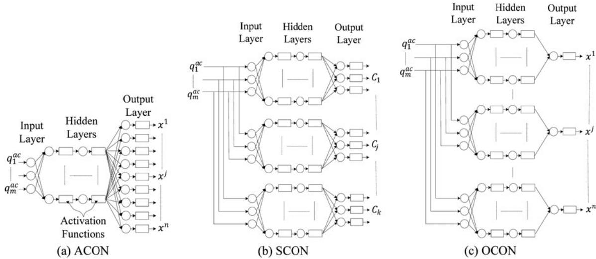
Figure 2. Schematic overview of (a) ACON, (b) SCON, and (c) OCON structures for ANNs.
