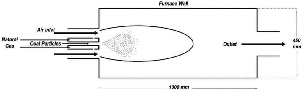
Fig. 1. Computational domain and furnace geometry.
