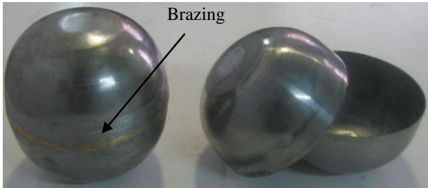
Fig 2. Manufactured hemi-spherical by two semi-sphericals.
