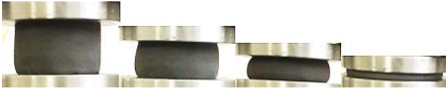
Fig. 2: deformations level of foam specimen.
