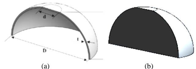
Fig. 1: Cut view of specimens. (a) Aluminum semi sphere. (b) Aluminum semi sphere with foam.
