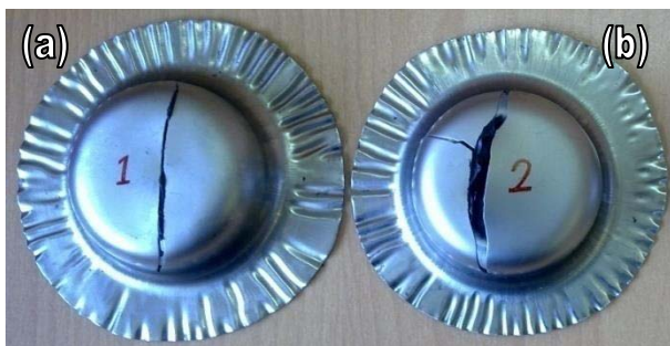
Figure 10. Tearing in the central area of cup for St 304 layer in (a) Al 1050/SUS sample (BHF = 17 kN, T = 100°C), and (b) Al 5052/SUS sample (BHF = 19 kN, T = 100°C).
