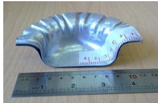
Figure 7. The section formed cup sectioned for evaluation of thickness strain.
