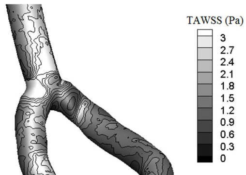
Fig. 6 Time average wall shear stress in vertebrobasilar system for a 20 year old man
