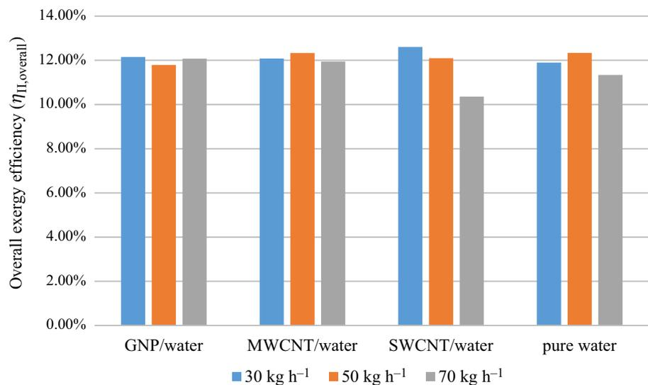
**Fig. 6** Overall energy efficiency in various mass flow rates in the average climate condition of 12:30 p.m. over the days of August 15–September 15
