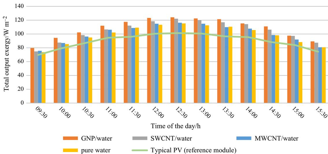
**Fig. 11** Average daily variations in the PVT total output exergy using different nanofluids and PV module (the tests are conducted from August 15 to September 15)
