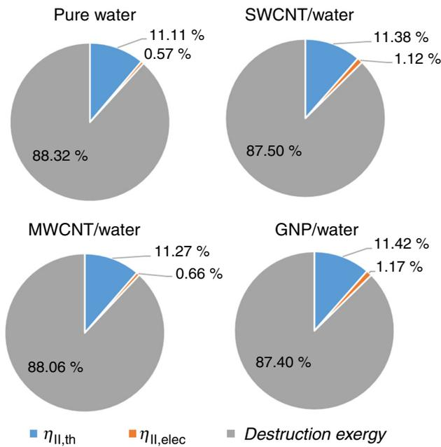
**Fig. 12** Average share of the different portions of input exergy for different working fluids (the tests are conducted from August 15 to September 15)
