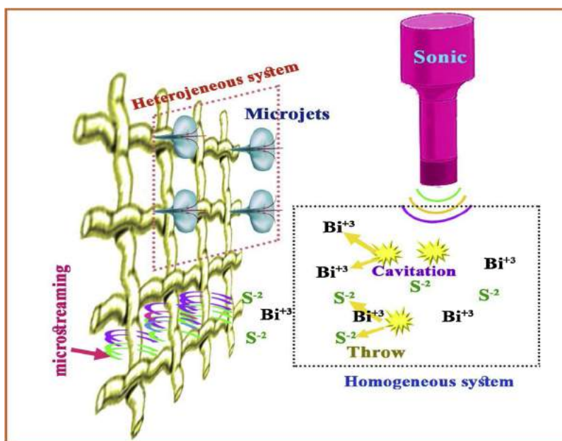
Fig. 6. Schematic presented the ultrasonic effects in sonodeposition process.
