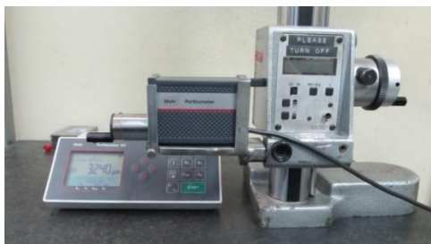
Fig. 2. The surface roughness tester used
