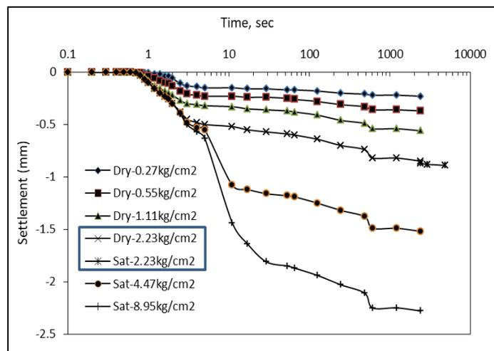
Figure 4. Settlement vs Time under Different Stress Levels with Half-Hour Soaking at 2.23kg/cm<sup>2</sup>.
