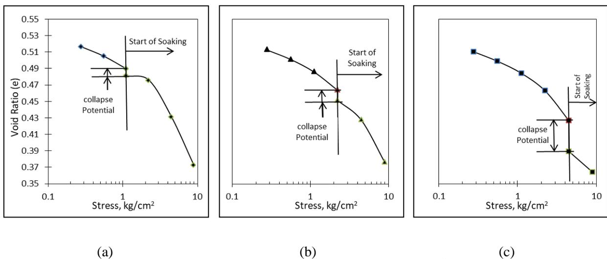
**Figure 10.** Void Ratio vs Stress with One-week Soaking at (a) 1.11kg/cm<sup>2</sup>, (b) 2.23kg/cm<sup>2</sup> and (c) 4.47kg/cm<sup>2</sup>.
