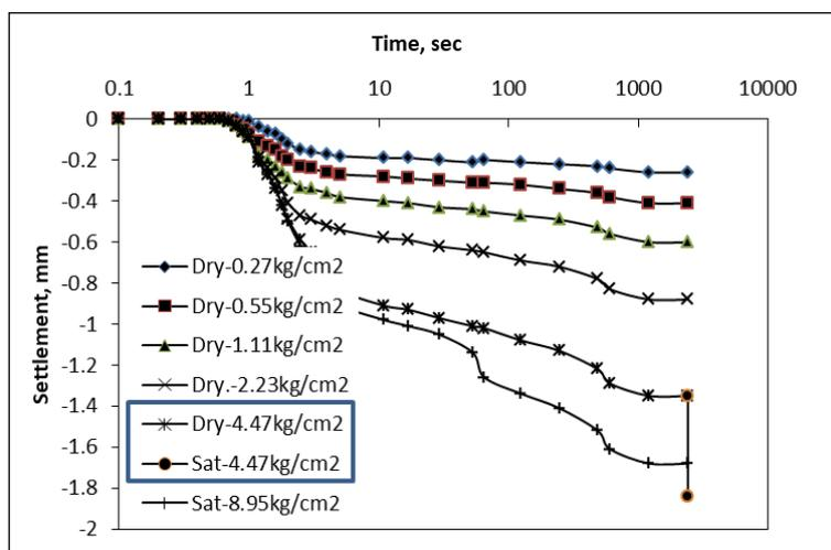
Figure 8. Settlement vs Time under Different Stress Levels with One-Week Soaking at 4.47kg/cm<sup>2</sup>.
