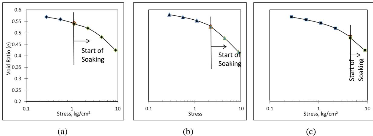
**Figure 9.** Void Ratio vs Stress with Half-hour Soaking at (a) 1.11kg/cm<sup>2</sup>, (b) 2.23kg/cm<sup>2</sup> and (c) 4.47kg/cm<sup>2</sup>.
