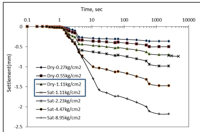
Figure 3. Settlement vs Time under Different Stress Levels with Half-Hour Soaking at 1.11kg/cm<sup>2</sup>.
