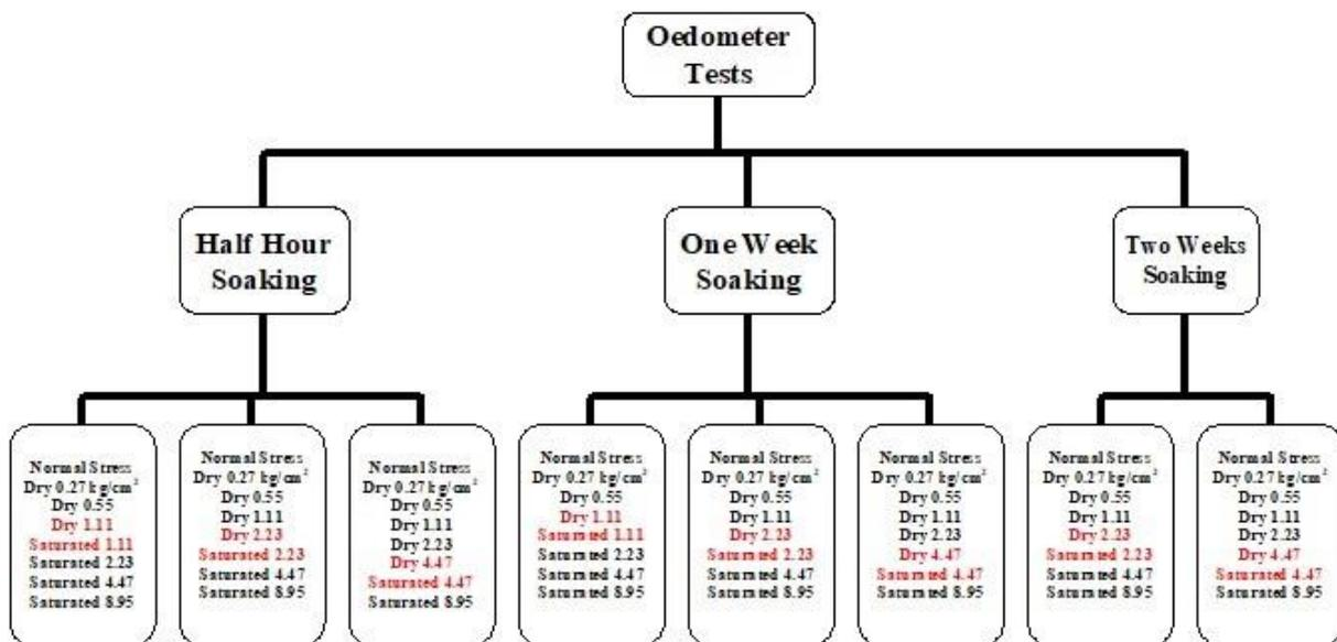
Figure 2. Program of Oedometer Tests.
