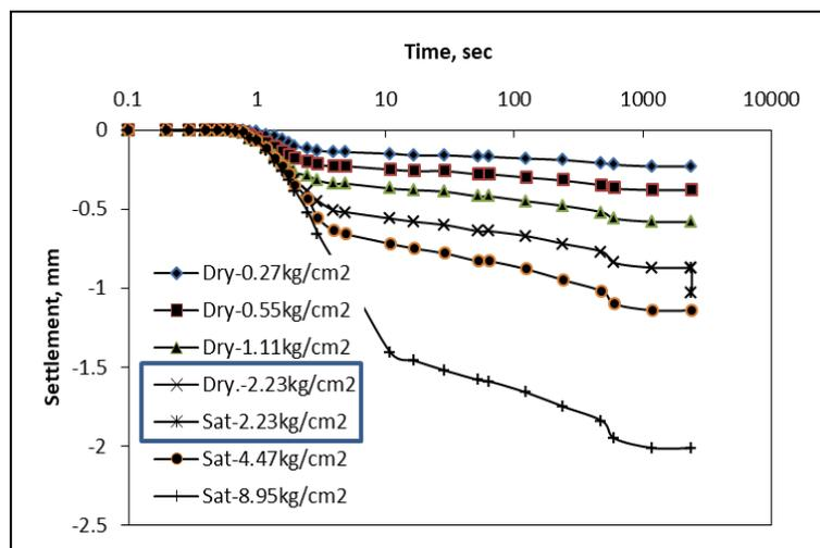
Figure 7. Settlement vs Time under Different Stress Levels with One-Week Soaking at 2.23kg/cm<sup>2</sup>.
