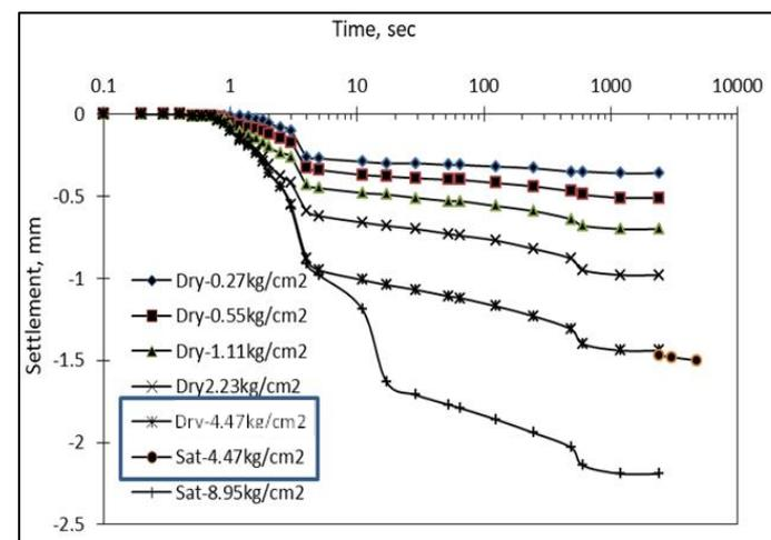
Figure 5. Settlement vs Time under Different Stress Levels with Half-Hour Soaking at 4.47kg/cm<sup>2</sup>.
