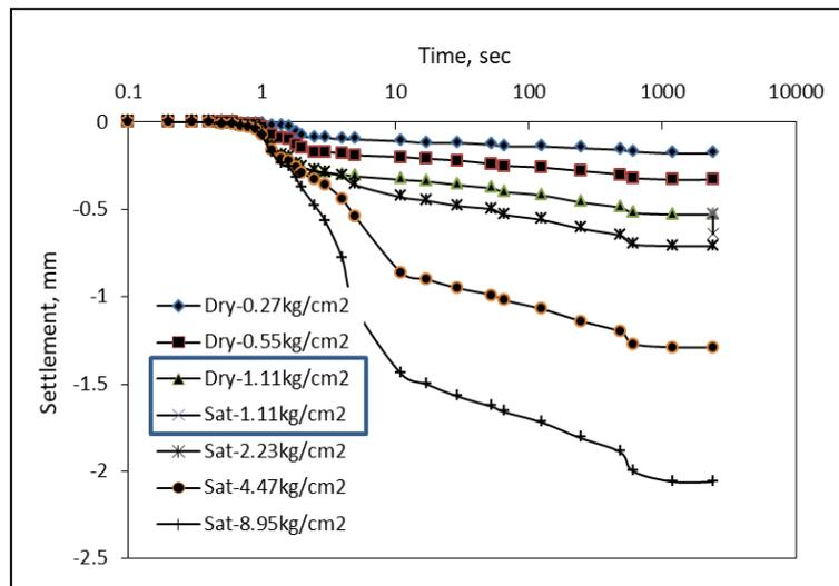
Figure 6. Settlement vs Time under Different Stress Levels with One-Week Soaking at 1.11kg/cm<sup>2</sup>.
