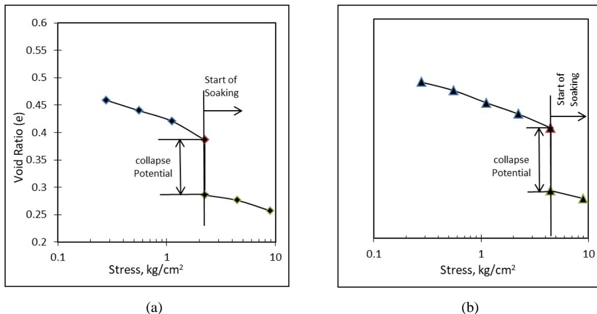
**Figure 11.** Void Ratio vs Stress with Two-Week Soaking at (a) 2.23kg/cm<sup>2</sup> and (b) 4.47kg/cm<sup>2</sup>.
