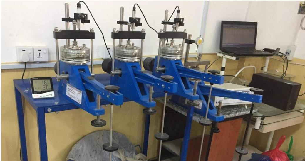
Figure 1. Multi-Cell Computerize Oedometer.
