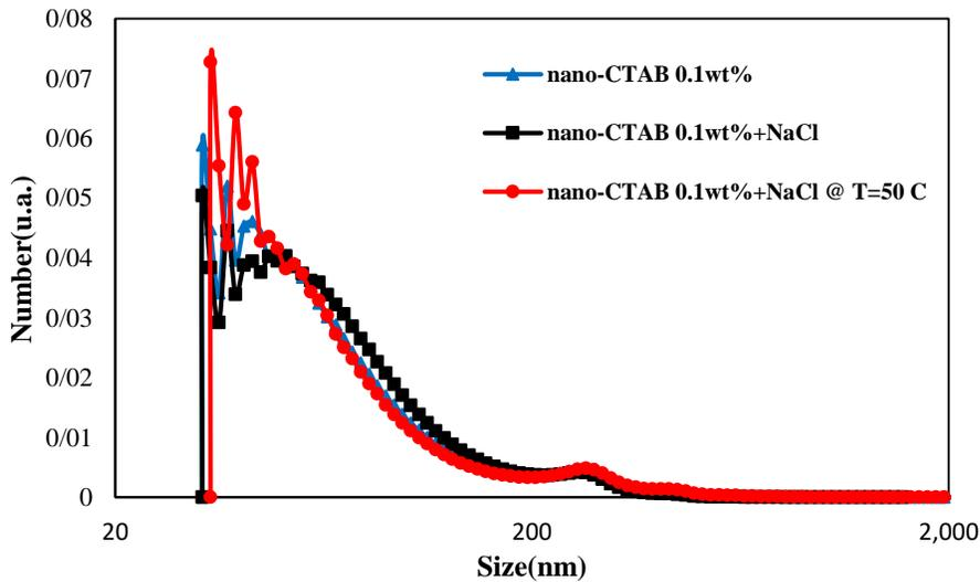
Figure 4. Particle size of nano-CTAB at 1 wt% at different salinity and temperatures.
