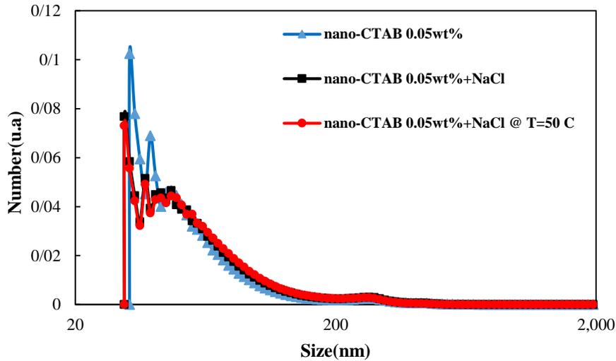
Figure 3. Particle size of nano-CTAB at 0.05 wt% at different salinity and temperatures.
