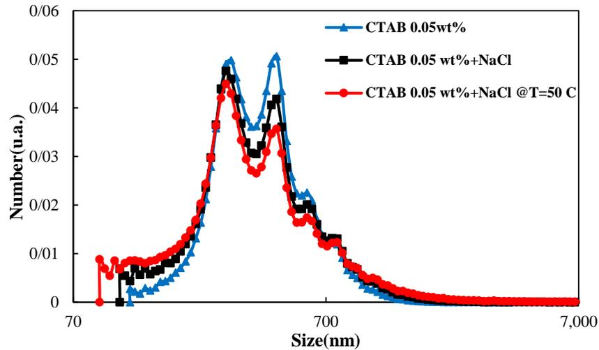
Figure 1. Particle size of CTAB at 0.05wt% at different salinity and temperatures.
