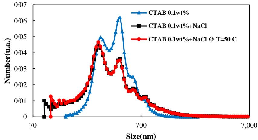
Figure 2. Particle size of CTAB at 0.1wt% at different salinity and temperatures.
